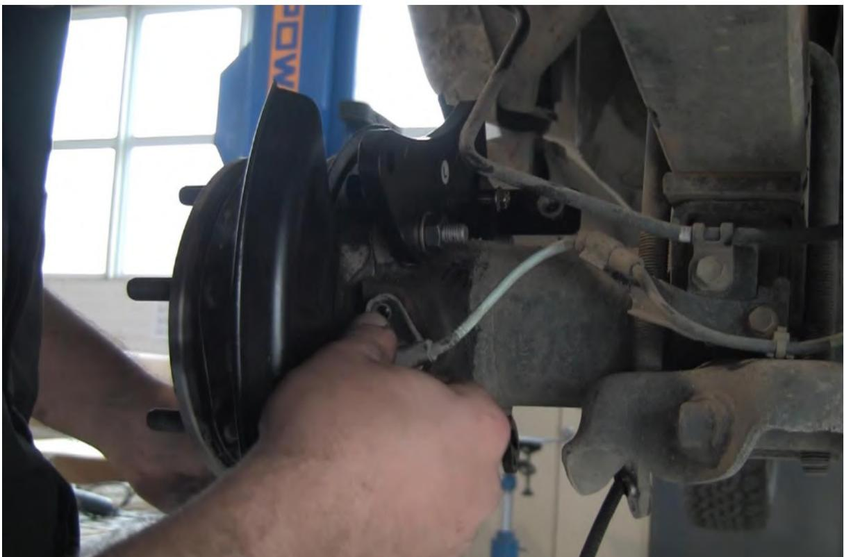
Refit handbrake assembly and hand brake cable onto the backing plate. #9 & #22
