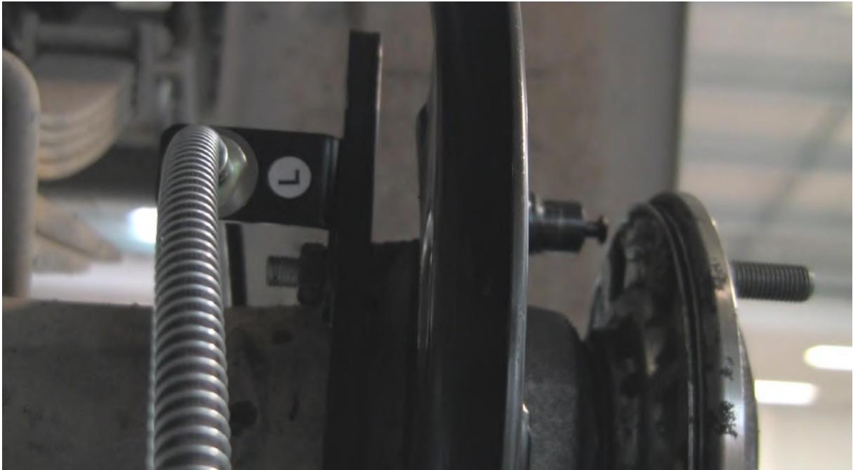
Refit the ABS sensor into the housing, making sure the area is clean.
