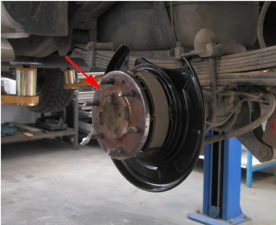
Fit the new brake rotor.
