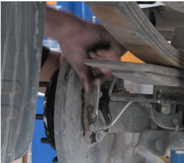
Remove the handbrake retaining clip and cable.
