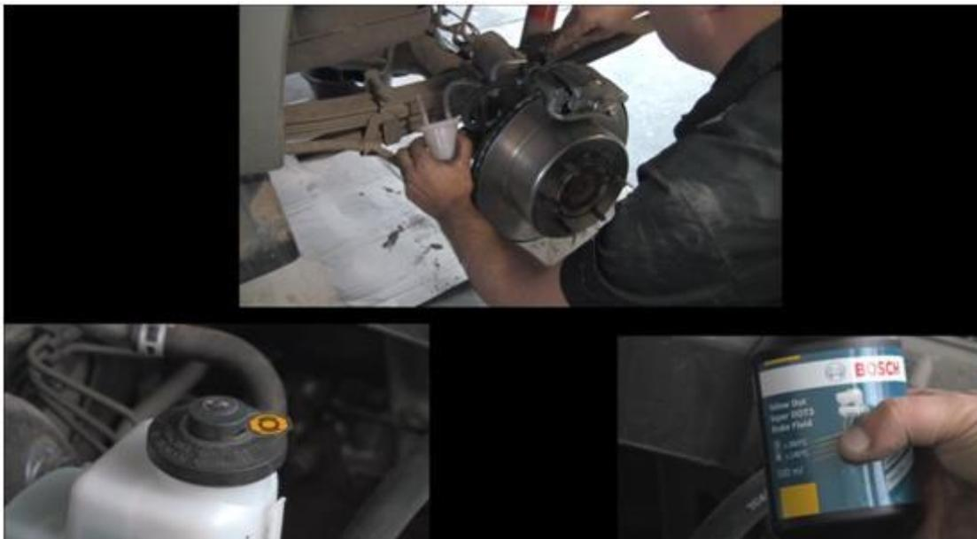
Adjust the handbrake shoes to the required tension via the access port in the backing plate. #20
