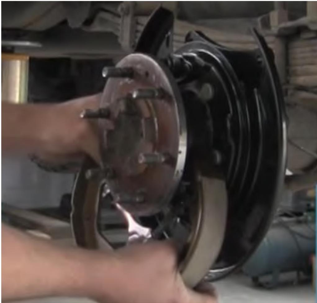
Refit the brake line to the new mount. #15
