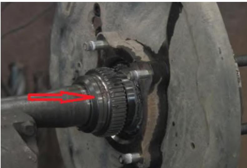
Knock out the four studs from the axle bearing housing.
