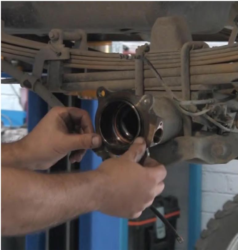
It is critical to ensure that the inner axle seal contacts the centre of the axle collar.
