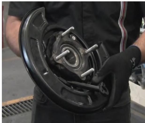
Take the assembly back to the press and press the axle into the hub.
