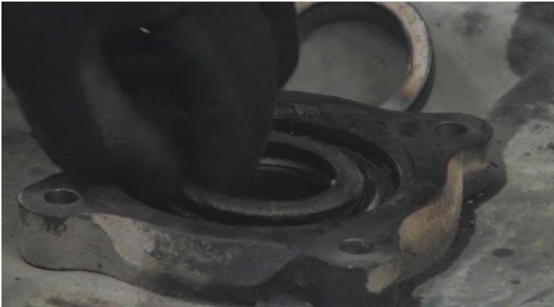
Remove the housing from the backing plate and using a press, remove the old wheel bearing.
