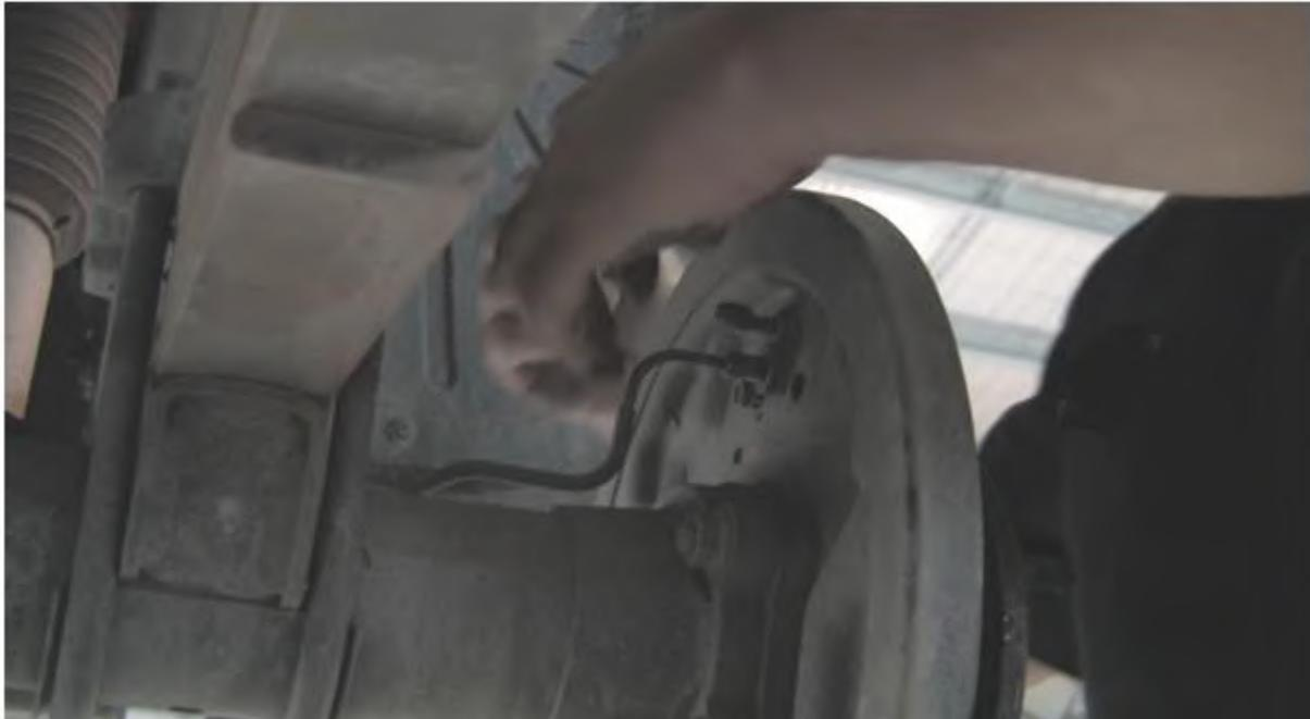
Carefully remove the ABS sensor and place it out of way.
