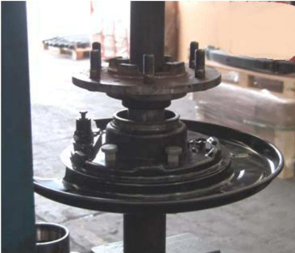
Return assembly to the bench vice and refit lock washer and axle bearing nut.
