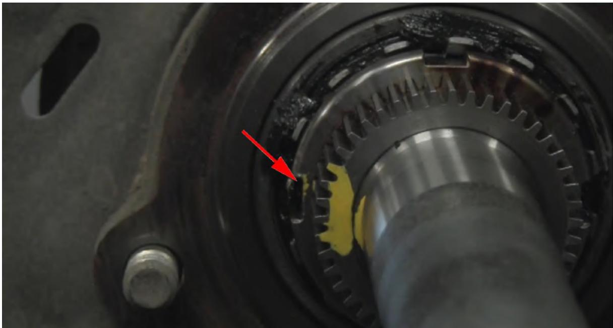
Knock out the four studs from the axle bearing housing.
