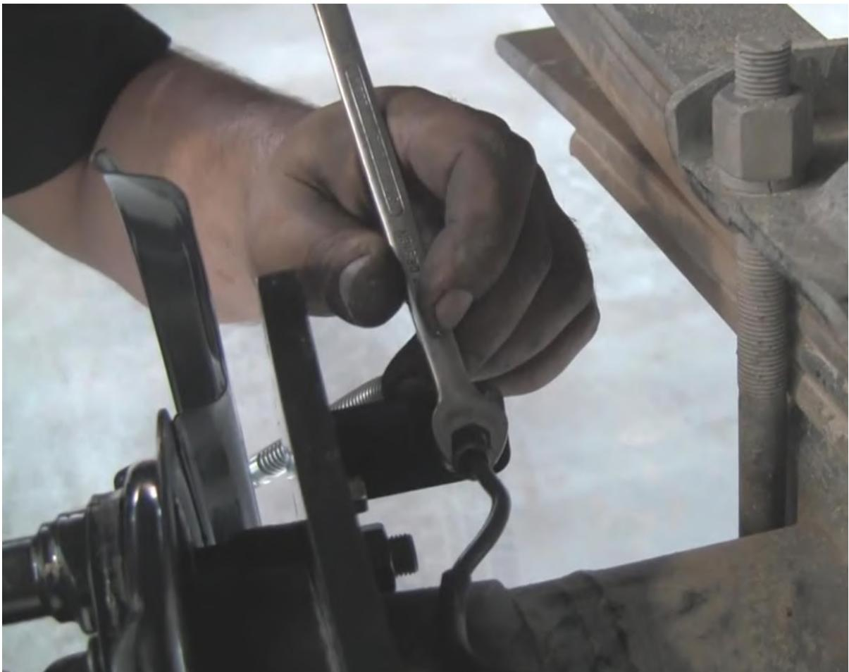
Fit the new handbrake assembly and refit the cable. #9 & #22
