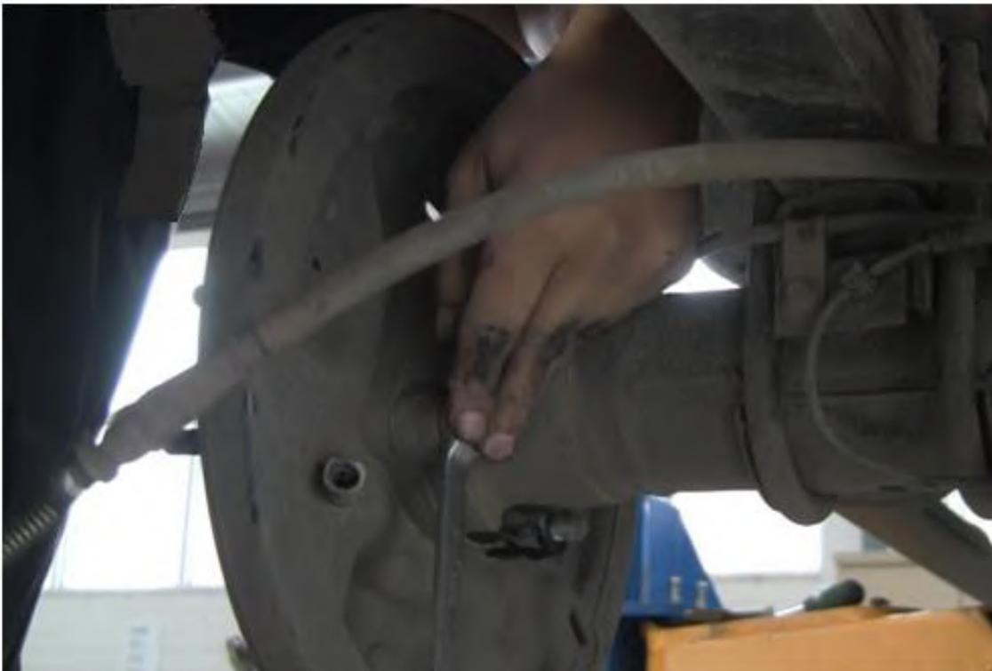
Remove the axle from the vehicle.
