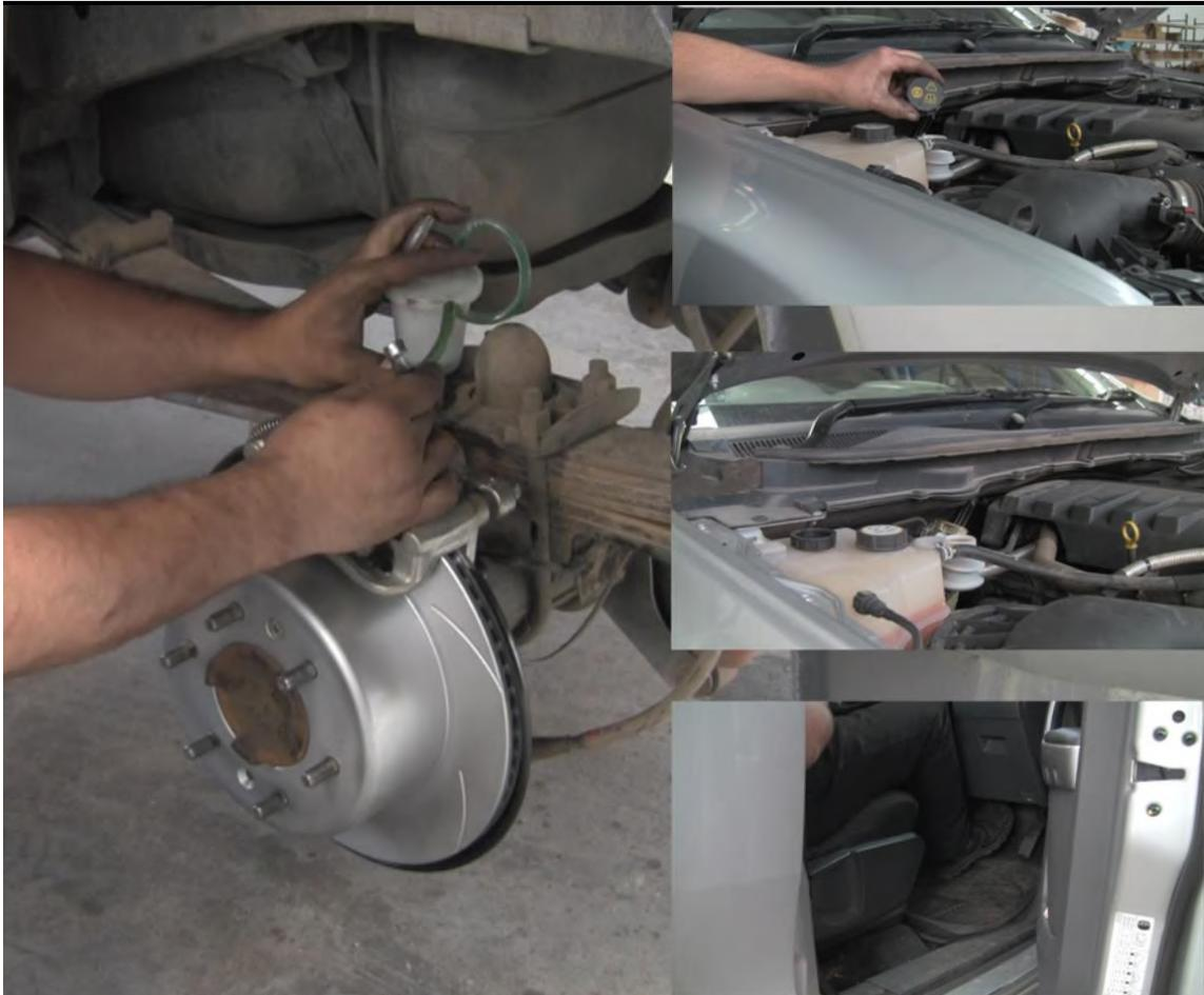
Adjust the handbrake shoes to the required tension via the access port in the backing plate. #20
