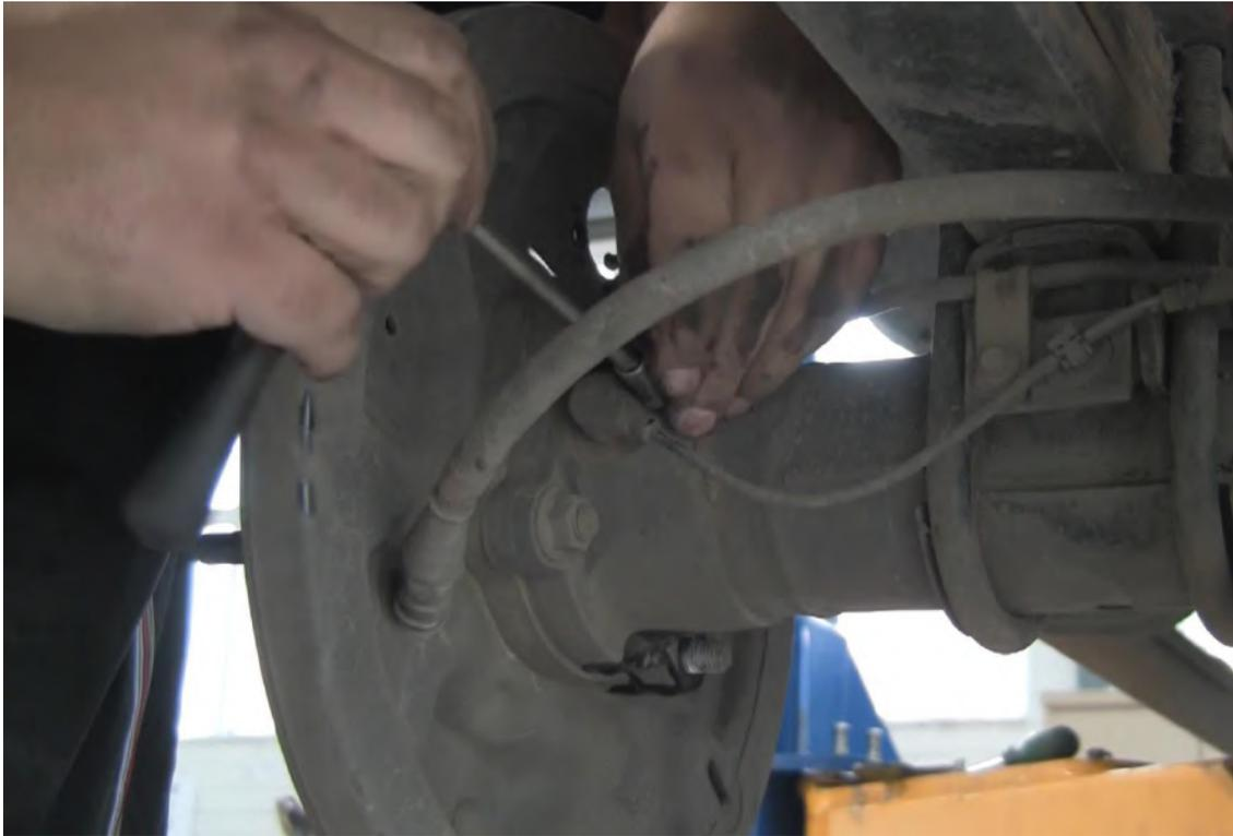
Remove the handbrake retaining clip and cable.
