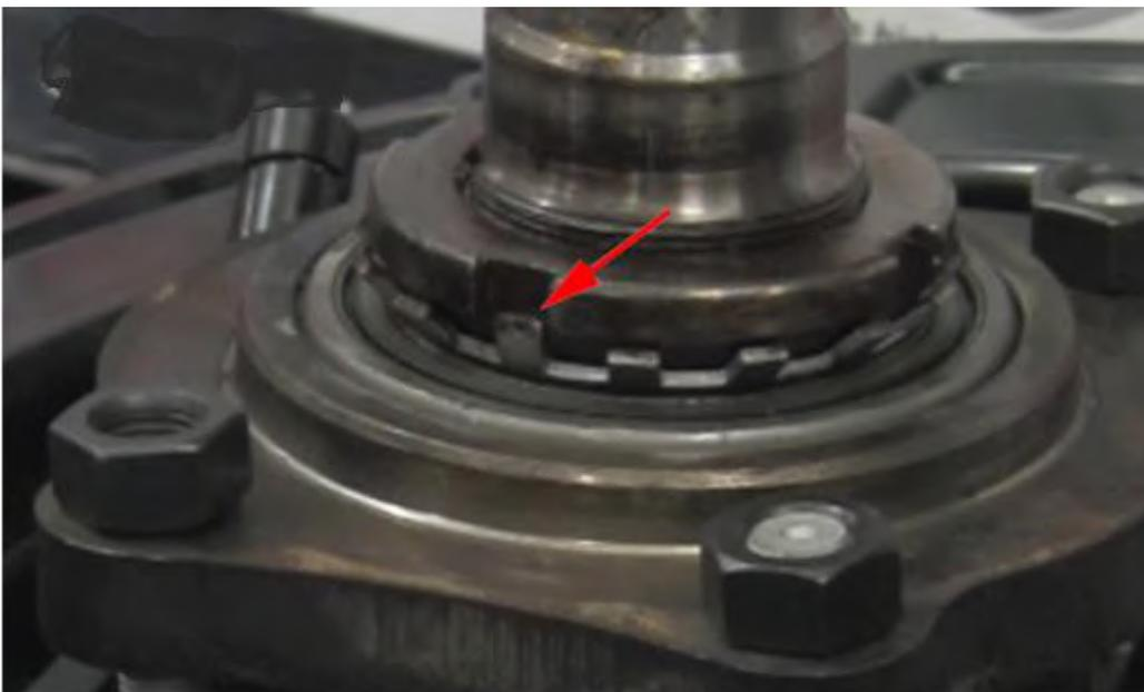
Press the ABS ring onto the axle.
