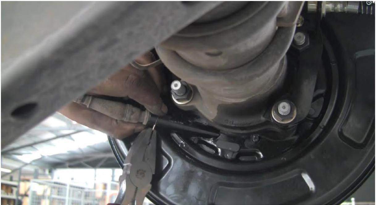
Refit the brake line to the new mount. #15
