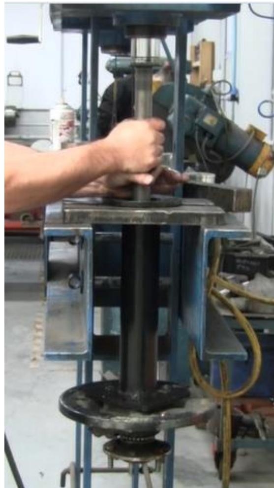
Then remove the bearing from the housing.
