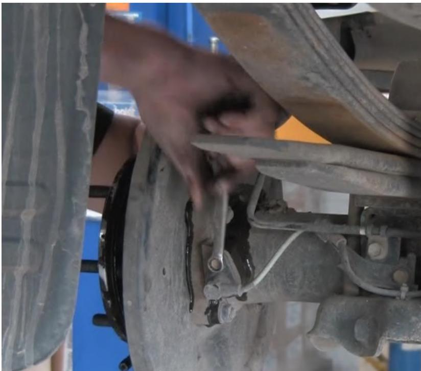
Remove the handbrake retaining clip and cable.
