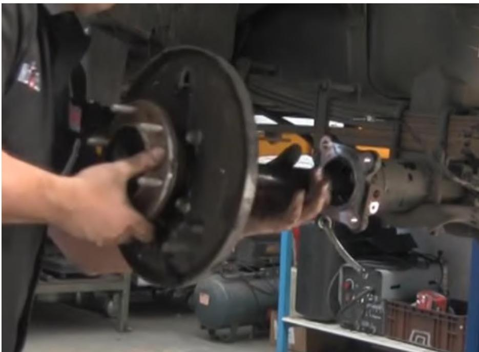
Remove the circlip, holding the tone wheel.
