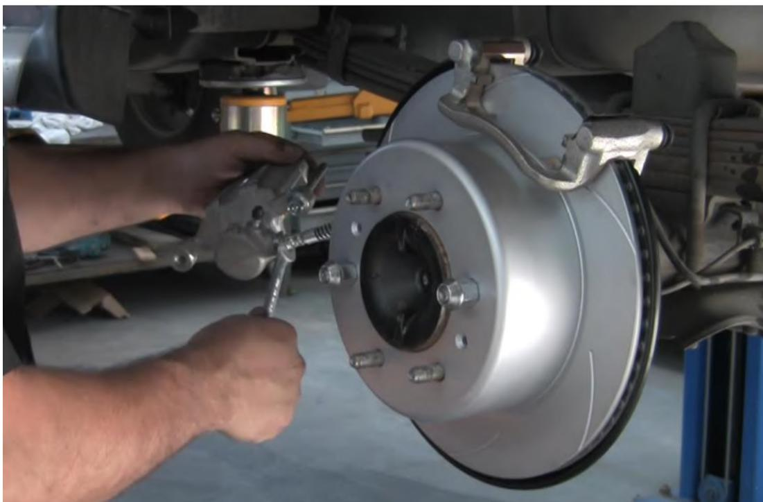
Bolt the caliper into the cradle with retaining bolts and tighten.
