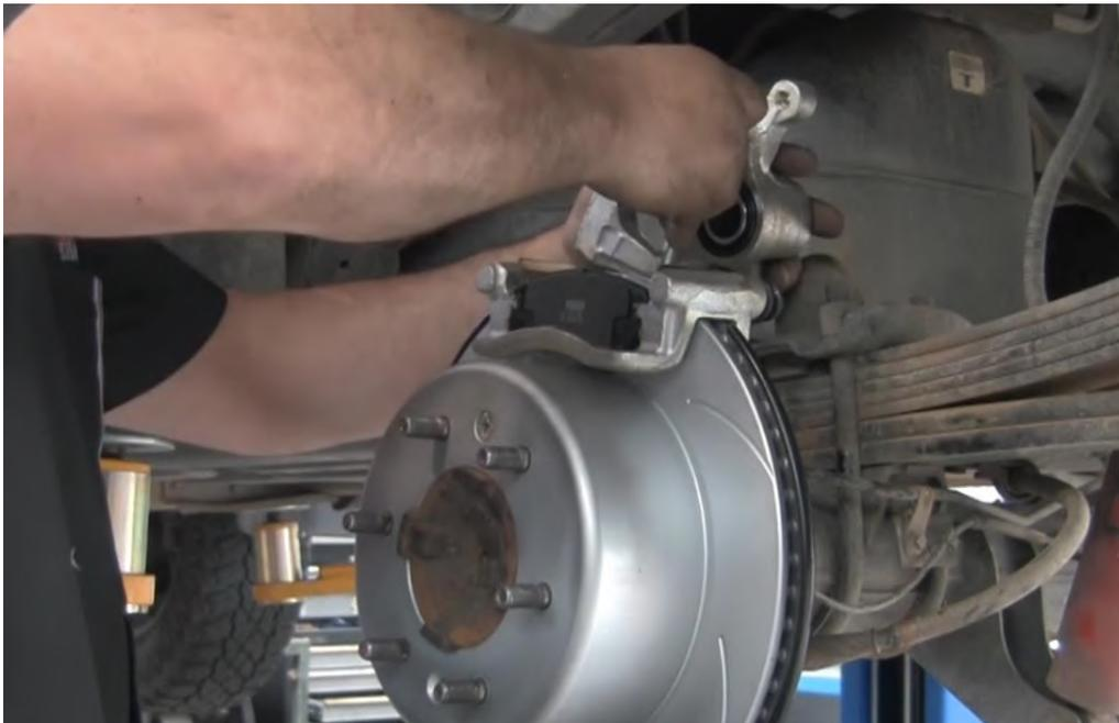
Recheck all bolts are to the correct torque.
