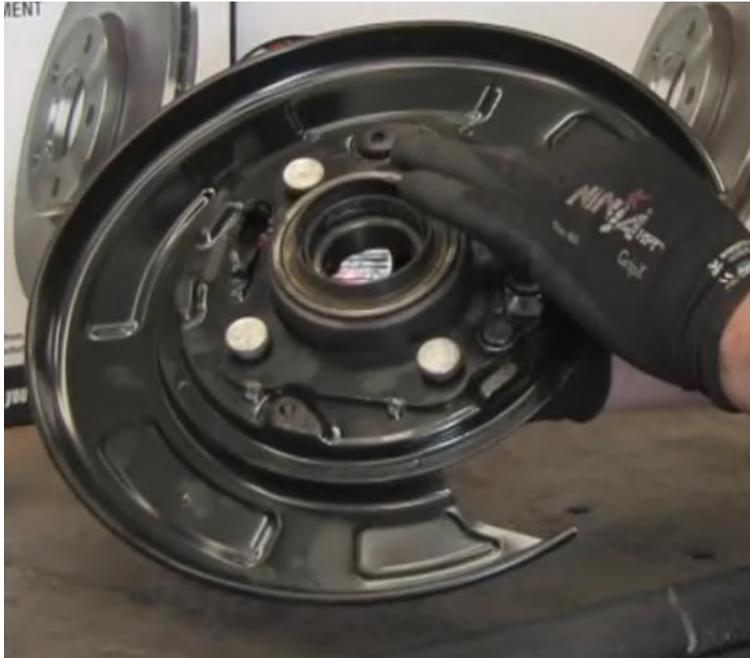
Place the inner bearing race onto the bearing housing and then the completed assembly onto the axle. Use the press to complete the operations.
