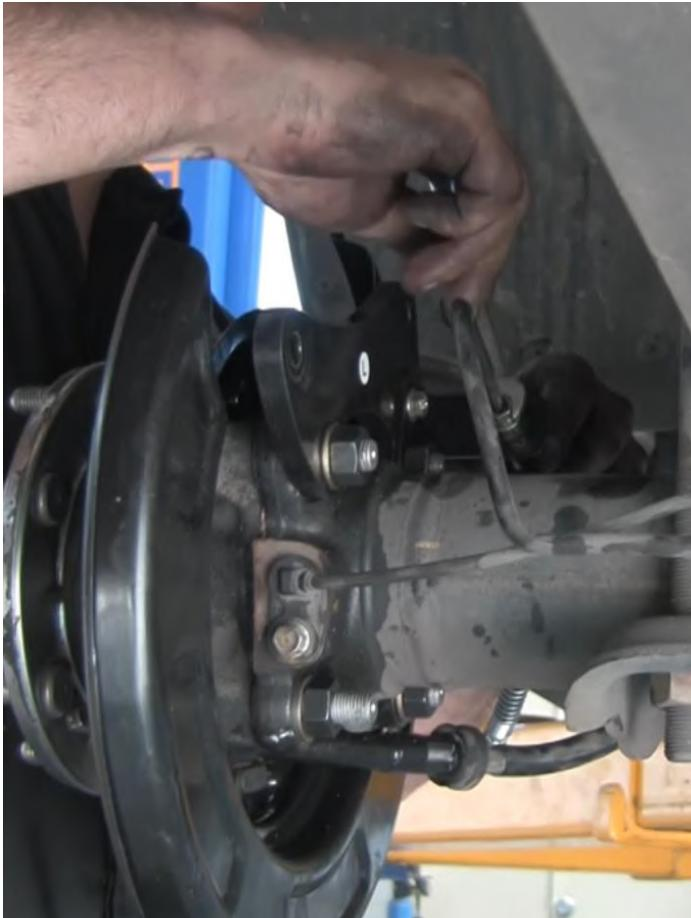
Before fitting the new brake rotor, make sure the axle face is clean.
