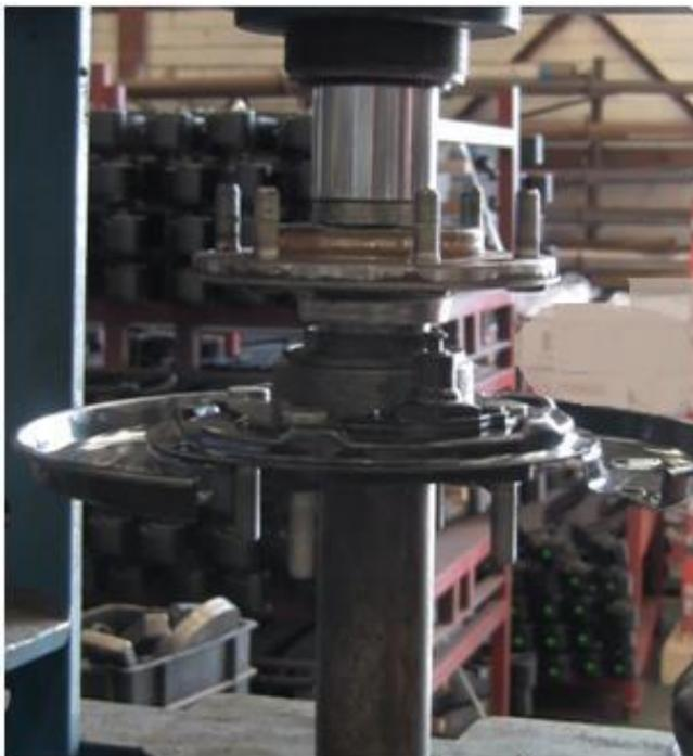
Press the supplied ABS tone ring into place with the same orientation as the original.
